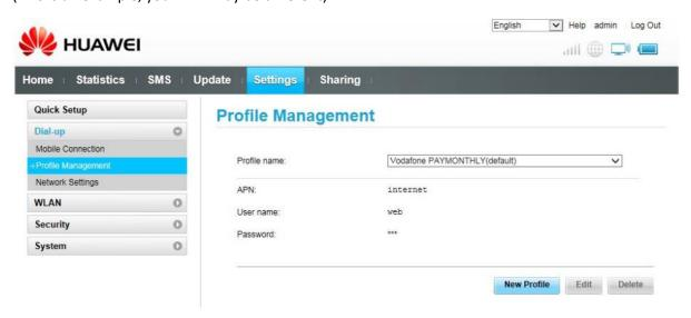
Check the APN profile that is applied, it should match the instructions sent with the SIM.
